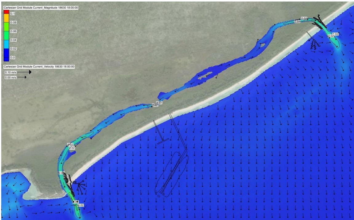
Figure 6. Scenario 1 (Tide Forcing Only) Current Velocity Outputs (m/s) During a Typical Falling Tide
